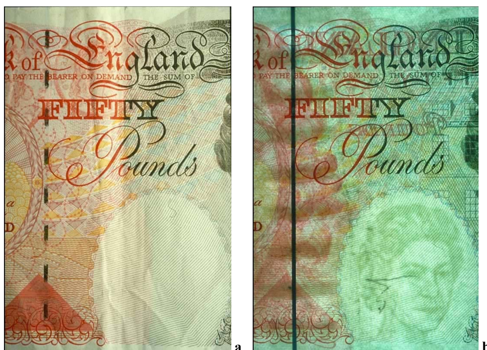
Figure 4 - The windowed thread on a genuine UK £50: (a) in diffuse reflection, and (b) in transmission (note the watermark bar pattern).
