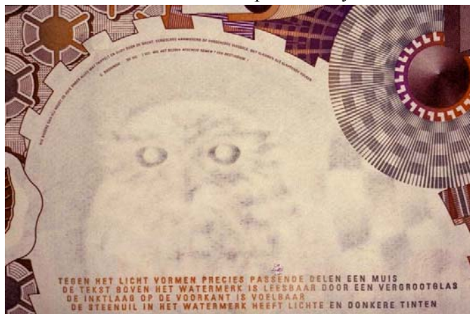
Figure 2 - Mould made watermark in the DFL 100 note, showing image elements that are darker and lighter than the background.
