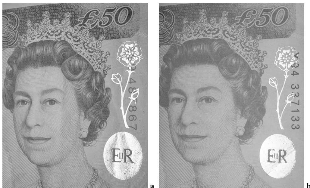
Figure 7 - Aluminium foil printing on a UK £50 note: (a) genuine note, and (b) counterfeit note printed in offset.
