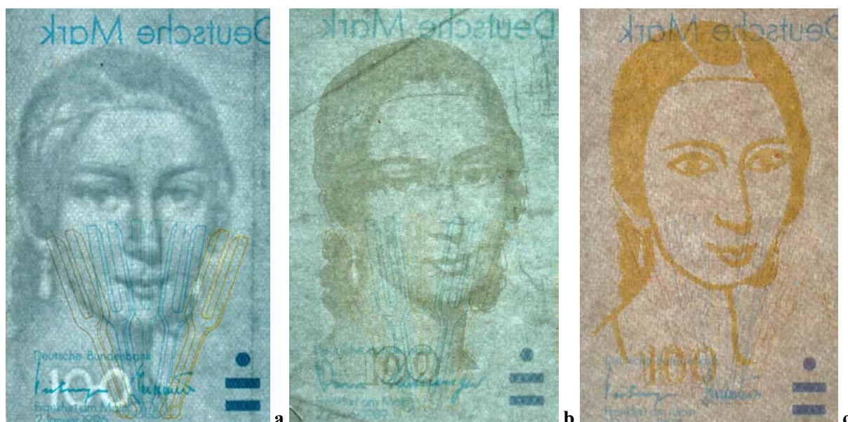
Figure 3 - watermark in DM 100 note: (a) authentic watermark, (b) half tone imitation, (c) single tone imitation.
