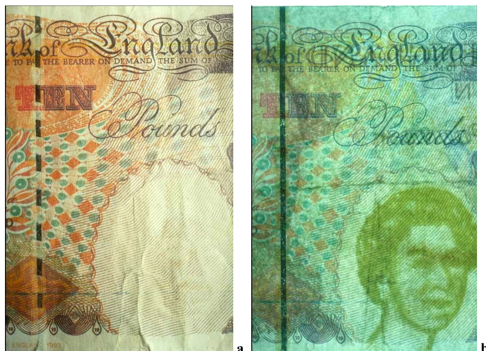
Figure 5 - Counterfeit UK £10 with imitation windowed thread: (a) in diffuse reflection, (b) in transmission (note the absence of the watermark bar pattern).
